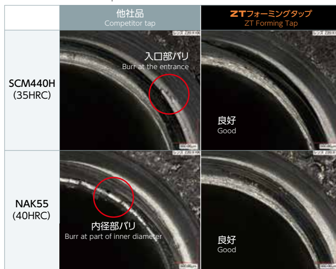
めねじのバリ比較 Comparison of internal threads burr
