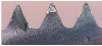
従来品 10穴加工後 Conventional after threading 10 holes.
