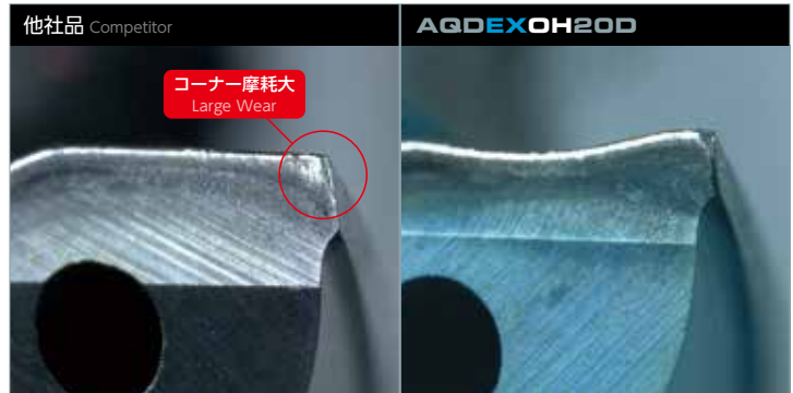
1350穴加工後摩耗比較 Comparison of wear after 1350 hole drilling
